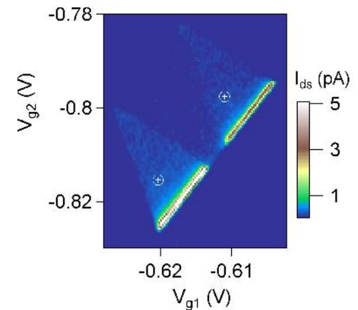
Fig. 3: Experimental signature at 100mK of a Coupled-Atom transistor in which transport occurs via two dopant's orbitals in series. This allows to perform spectroscopy, electron pumping and probe coherence. **Phys. Rev. Lett. 108, 206812 (2012)**
