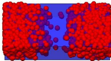
Fig. 2: Single-Atom transistor using dopant diffusion in a very small CMOS transistor channel volume. **Nature Nanotech. 5, 133 (2010)**
