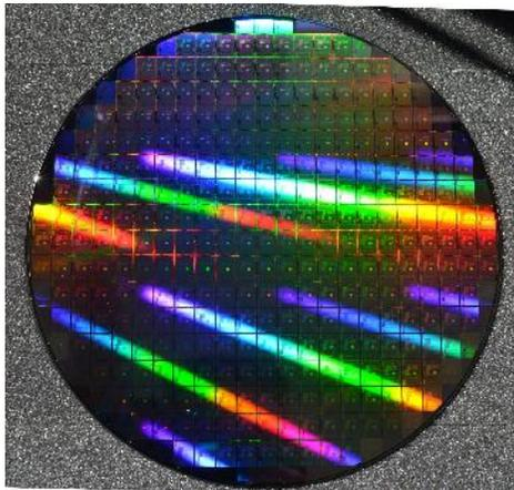
Fig1: 300mm wafer using trigate SOI technology, with SATs and CATs. collaboration CEA-INAC & CEA-Leti
